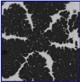
*Fig. 1. Microstructure of an alloy from a binary alloy system that features a retrograde solidus line (Ag-Bi); primary dendrites were partially remelted due to supersaturation occurring upon cooling.*
