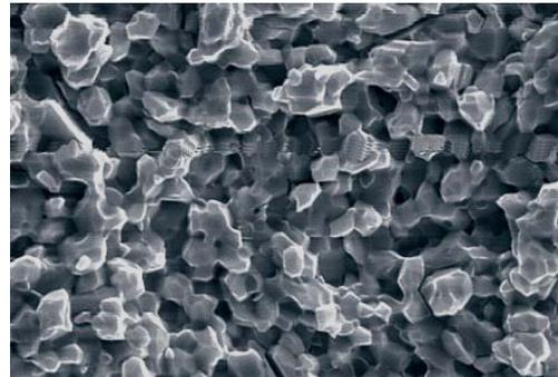
*Fig. 2: Fracture surface of a solder alloy wire of Zn-Al-Ga, after extrusion embrittled due to supersaturation that occurs in the fcc (Al) phase.*
