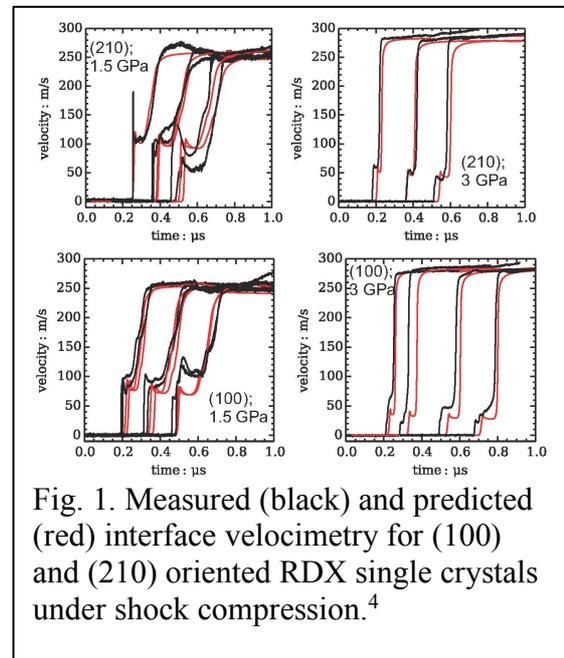
Fig. 1. Measured (black) and predicted (red) interface velocimetry for (100) and (210) oriented RDX single crystals under shock compression.<sup>4</sup>
