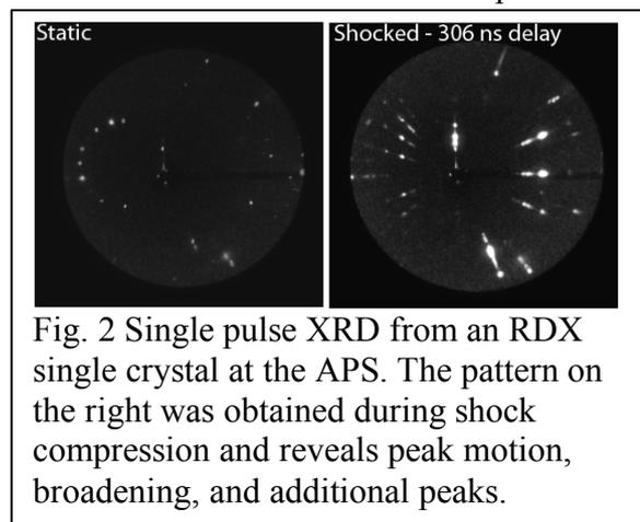
Fig. 2 Single pulse XRD from an RDX single crystal at the APS. The pattern on the right was obtained during shock compression and reveals peak motion, broadening, and additional peaks.
