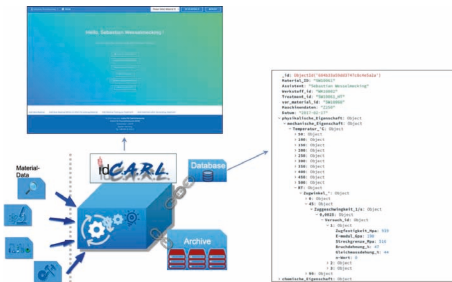
Fig. 12.2: Schematic representation of idCarl as data transformer: Processing of material data from experiments.
