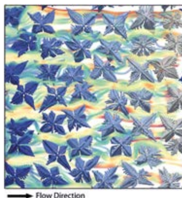
View from the top of the simulation domain depicting stream lines of a flow through a channel along dendrites.
