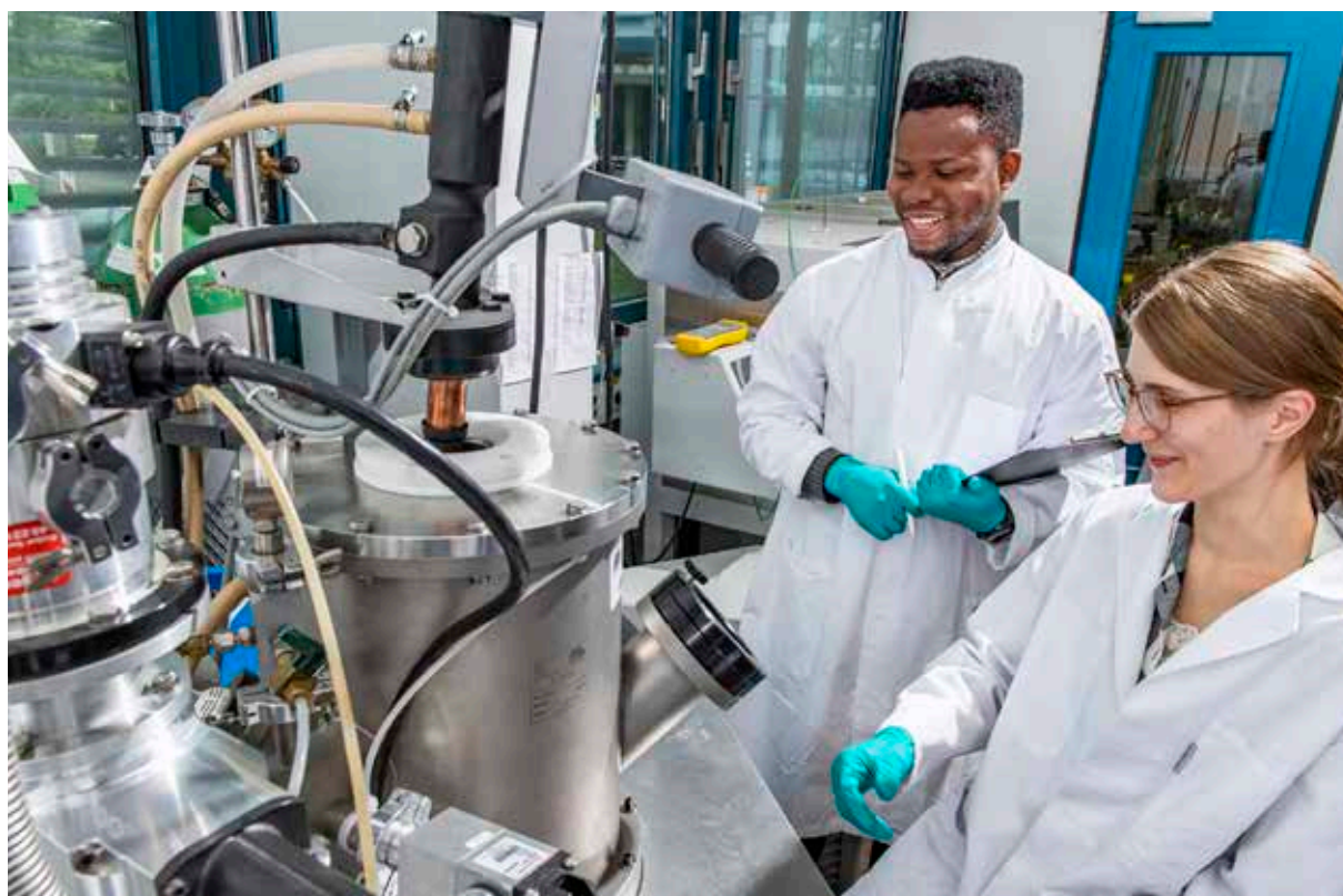
Fig. 11.1: Arc melting. Hannah Mittag and former MSS student Oluwaseyi Oluwabi preparing alloys for research on chemically complex shape memory alloys.
