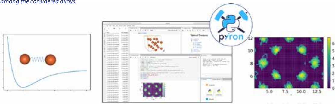
Fig. 10.3: By using the integrated development environment pyiron, the modelling strategies become easily readable in interactive notebooks (middle). They provide a direct link to the physical concepts and raw data (left) as well as to the final results appearing in publications (right).
